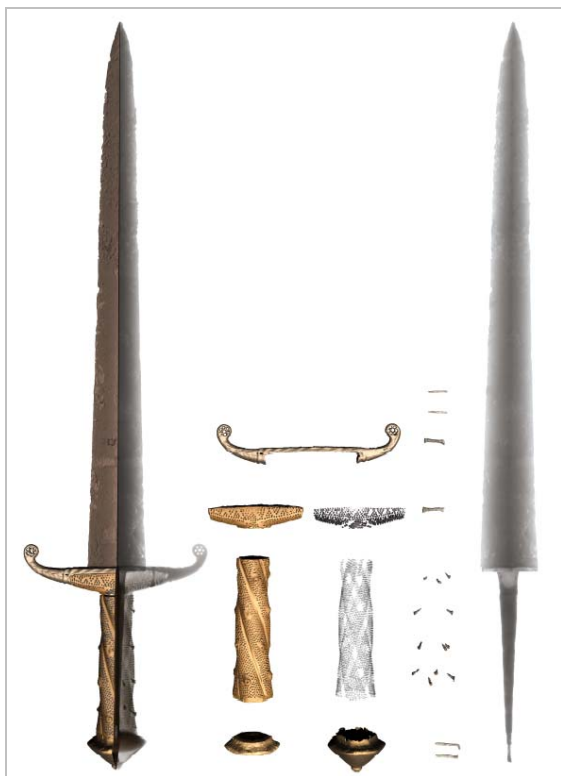
Fig. 8. 3D-visualisation of the combined X-ray and neutron CT data sets of a short sword (Zug, 15 th c., Switzerland); information of the small metal pieces such as ornaments pins and nails originate from the X-ray CT; the wooden parts and larger metal parts originate from the neutron CT. (from Mannes et al. (2015); a YouTube video is accessible, too: NIAG - Neutron Imaging and Activation Group 2015)
