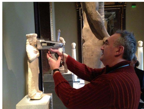
Fig. 2.: In situ application of a hand-held X-Ray Fluorescence analyser for the non-destructive examination of the traces of polychromy remained on the surface of ancient marble sculptures (Kunst Historisches Museum, Vienna, source: IAEA homepage)
