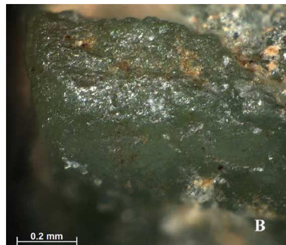
Fig. 15.: Stereomicroscopic images of chloritic rock (sample SM 9-14-10), a – texture in general, b – chlorite grains
