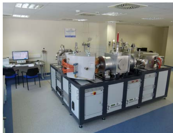
Fig. 3.: The MICADAS AMS system installed at Debrecen (courtesy Dr. M. Molnár).
