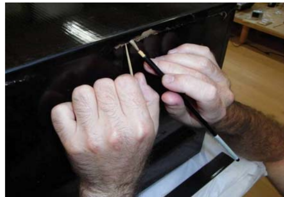
Fig. 15.: Application of adhesive mixture on the bottom box
