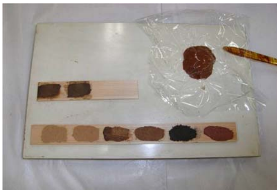
Fig. 16.: Test board of different filling mixtures with incense powder
