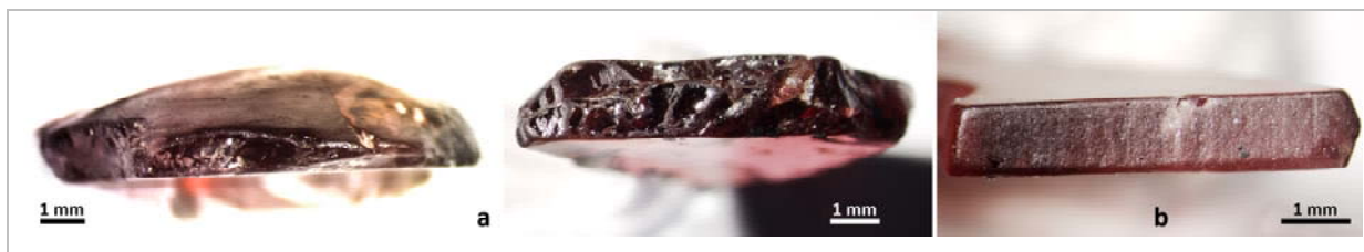
Fig. 5.: a) facet rough edges on two semi-finished pieces (No.2 and No.9) b) wheel-cut edges on a finished piece (No.15). Photo: Eszter Horváth
