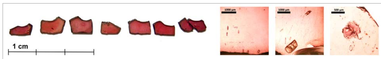
Fig. 12.: Garnet slices from Bezenye-Papré and their typical mineral inclusions: apatite and zircon crystals. Photo: Eszter Horváth
