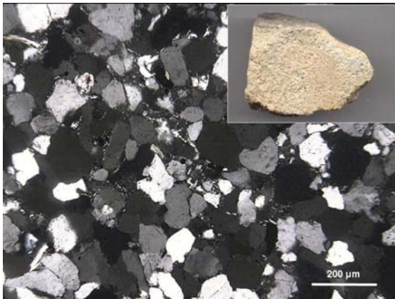
Fig. 14.: Mature, quartz rich sandstone in a hand specimen (upper right) and micrograph in polarized light
