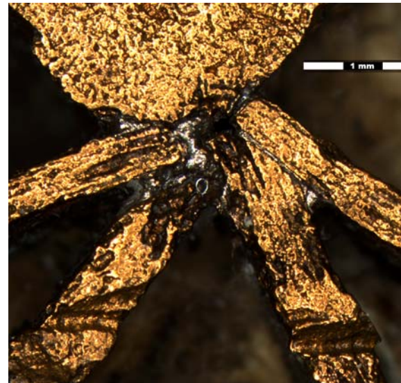
Fig. 9.: Soldering material at the joining point of cell walls
