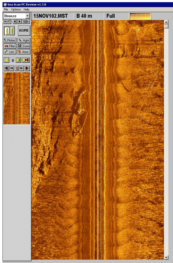
Figure 4. Side-scan sonar image of a modern ship, Wörthersee, Austria. (courtesy C. Dworsky)
