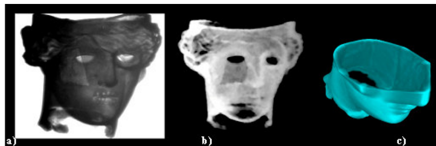
Figure 7. a) Greek Bronze Head b) Digital Radiography c) 3D elaboration
