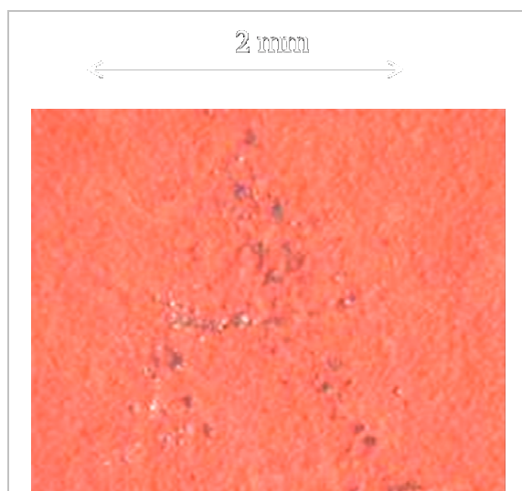
Figure 3. Track left by a Pb stylus on paper prepared using a mixture of cinnabar ( \text{HgS} ) and lead-white ( (2\text{PbCO}_3 \cdot \text{Pb}(\text{OH})_2) )
