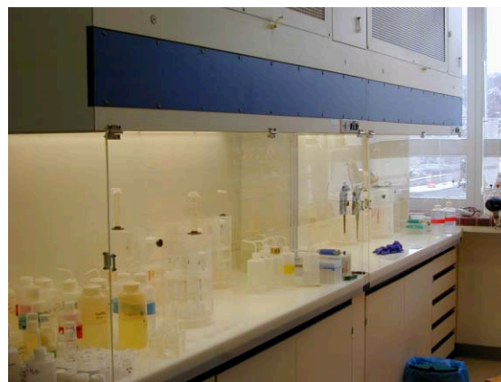
Fig. 3: One of the working benches in the geochemistry clean-lab at Tübingen University. In this laboratory the amount of air particles is reduced with filter systems to a minimum, the fume hood inside the lab provide even better conditions in order to avoid contamination of Sr (or Nd) from the sample to be analysed by other sources.
