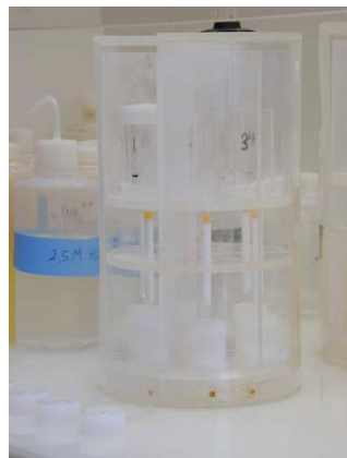
Fig. 2: Cation exchange chromatography resin in cigarette-like columns, designed especially to separate Sr from other elements. The carousel is placed in an ultra-clean fume hood in the clean lab.
