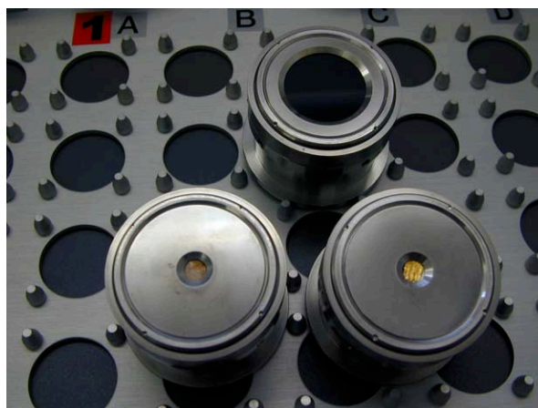
Fig. 5: Three XRF sample holders (closed, upside down), one with a conventional 34 mm window, the other two with 8 mm window, containing a rock-specimen (left) and a gold-foil (right) inside.
