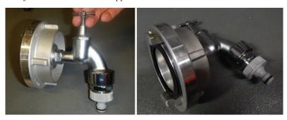
Picture 9–10: A hydrant faucet tool from a fire engine in Berlin, Germany Source: Photo taken by the author, 2019.
