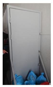
Picture 19: Installed or transportable practice door in the Central Fire Station, Haifa, Israel
