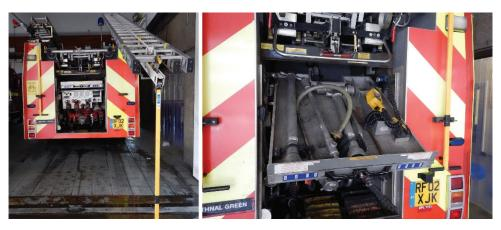
*Picture 12–13: Handles and lifted/tilted shelves for easier access of the fire equipment in London, United Kingdom*
