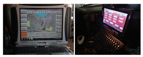
Picture 38–39: Special laptop and mobile terminal installed in fire trucks in Baltimore and Washington, D.C., United States
