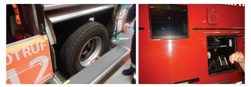
Picture 34–35: Using all spaces in a fire truck to install mobile steps in Berlin, Germany and outside control, display possibilities in a fire incident commander vehicle in Washington, D.C., United States
