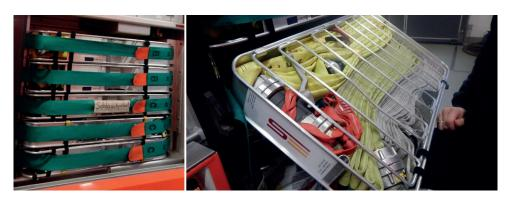
Picture 32–33: Prepared "fast attack" lines, hoses in a fire engine, and a solution with a tilted shelf for the easier accessibility Berlin, Germany
