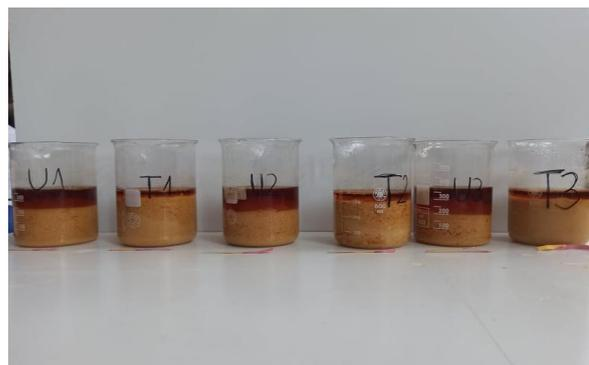
*Figure 4.* Separation of crystals by cooling at room temperature following the addition of urea and thiourea: U1, U2, U3 – samples to which urea was added; T1, T2, T3 – samples to which thiourea was added
