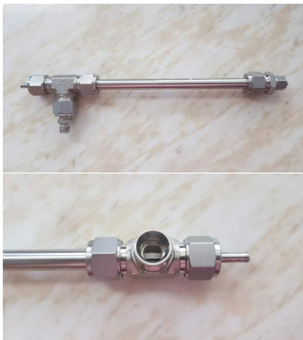
Figure 2: HC1 HF membrane mini-module
