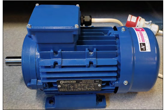
Figure 5. Electric motor for driving the generator.
