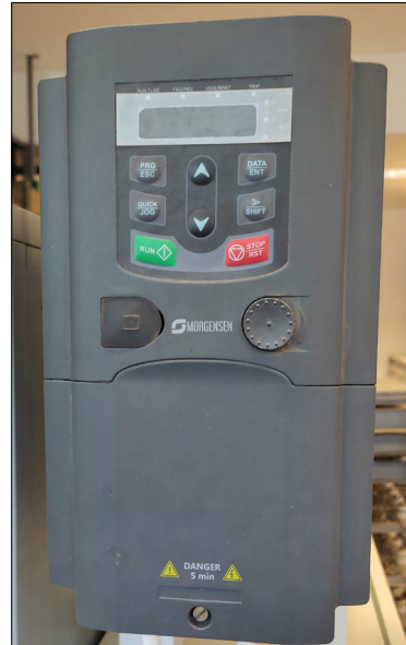
Figure 4. Morgensen MSI200A-004G/5R5P-4 frequency converter.
