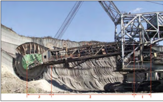
Figure 7. The load bearing structure of the BWE
