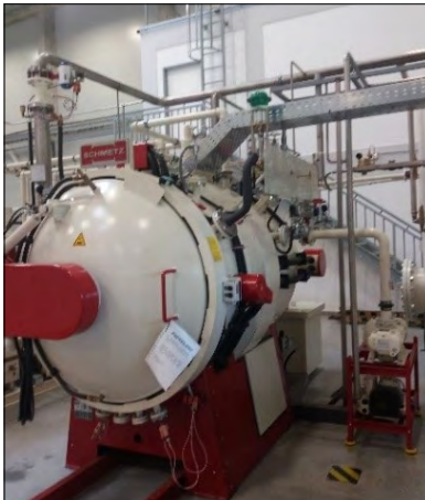
Figure 3. Schmetz vacuum furnace.
