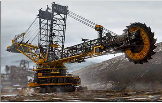
Figure 1. Bucket wheel excavator used in open pit coal mines.
