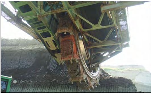
Figure 8. The bucket wheel in operation mounted on the boom
