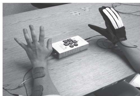
2.Figure. Contralaterally controlled functional electrical stimulation
