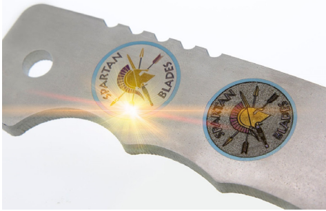
6. figure. Colour Laser Marking with FiberCube Laser Marking System
