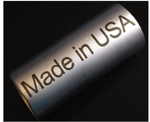
5. figure. Stainless Sleeve Laser Annealing.
