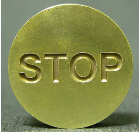
3. figure. Deep Laser Engraving in Brass for Elevator Buttons.
