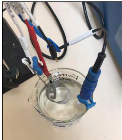
Figure 1. Corrosion measuring arrangement
