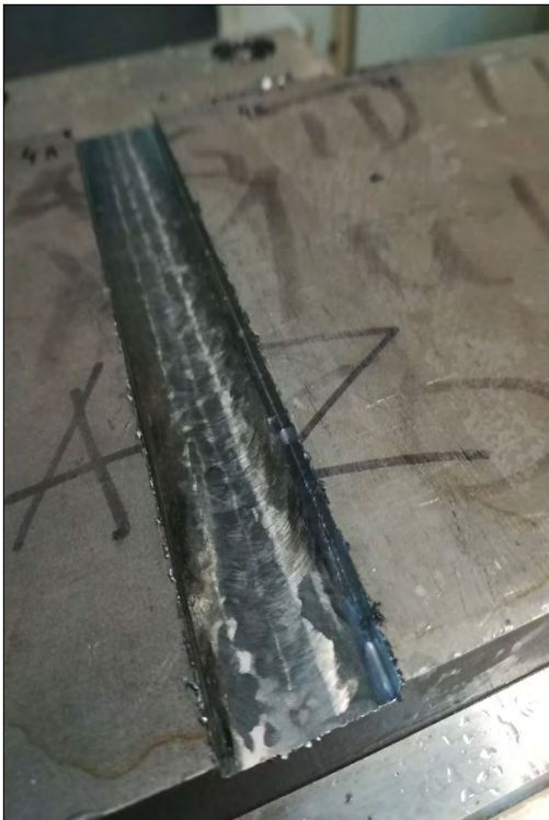
Figure 6. The AB1 groove's surface with protruding ragged edge (burr)
