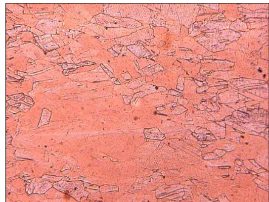
Figure 7. Copper microstructure linear magnification 50x, etched by ammonium hydroxide/hydrogen peroxide [7]
