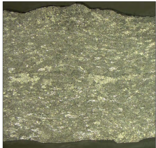
Figure 6. Cross section of the joint (aluminium sample)
