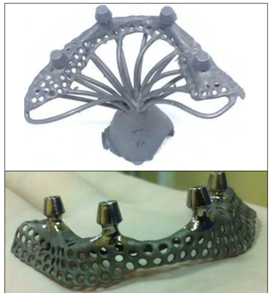
Figure 1. Raw cast of one-piece titanium metal structure, and the device ready to be implanted
