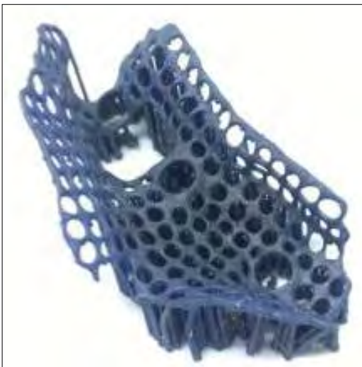
Figure 15. Base plate created with additive manufacturing (powder bed fusion), and the printed solid part with support structures
