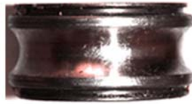
Figure 5. Failure of inner ring
