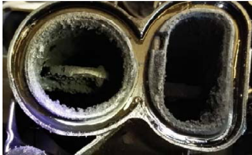
Figure 5. Oily soot deposits in the plastic intake pipe
