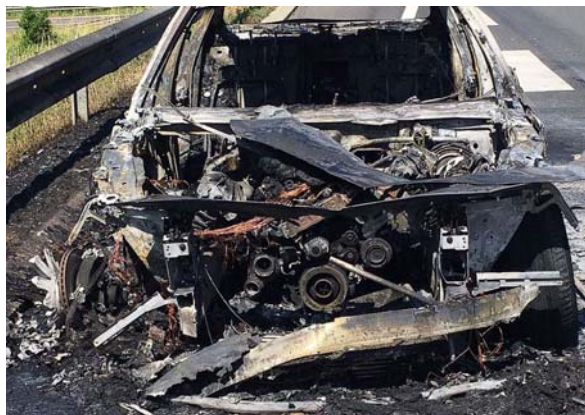
Figure 2. Vehicle with N47 engine after catching fire
