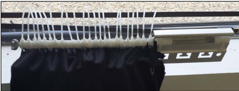
Figure 8. Wear-resistant plastic and connection between the rope and belt
