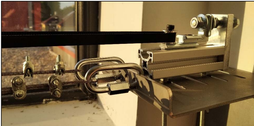
Figure 7. Stretching structure of ribbed belt
