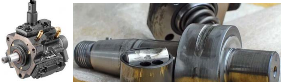
Figure 9. The high-pressure fuel pump, and wear resulting from the sticking of the piston, which results in the entry of metal dust into the system [BMW E91 N47 high pressure pump failure and repair, YouTube, source of picture]
