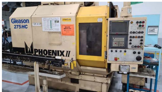
Figure 6. Phoenix II. second gen. 6 axis Gleason bevel gear cutter [source: internet]
