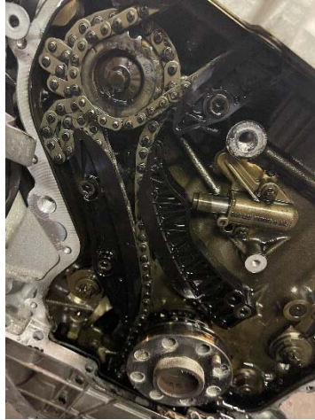
Figure 1. Timing chain failure (break)
