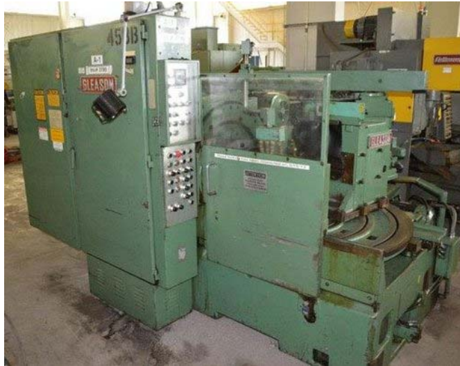
Figure 5. Gleason No.641 Generator (PLC controlled) [source: internet]
