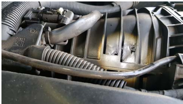
Figure 6. Melting of the cover on the engine as a result of the puncture of the intake pipe
