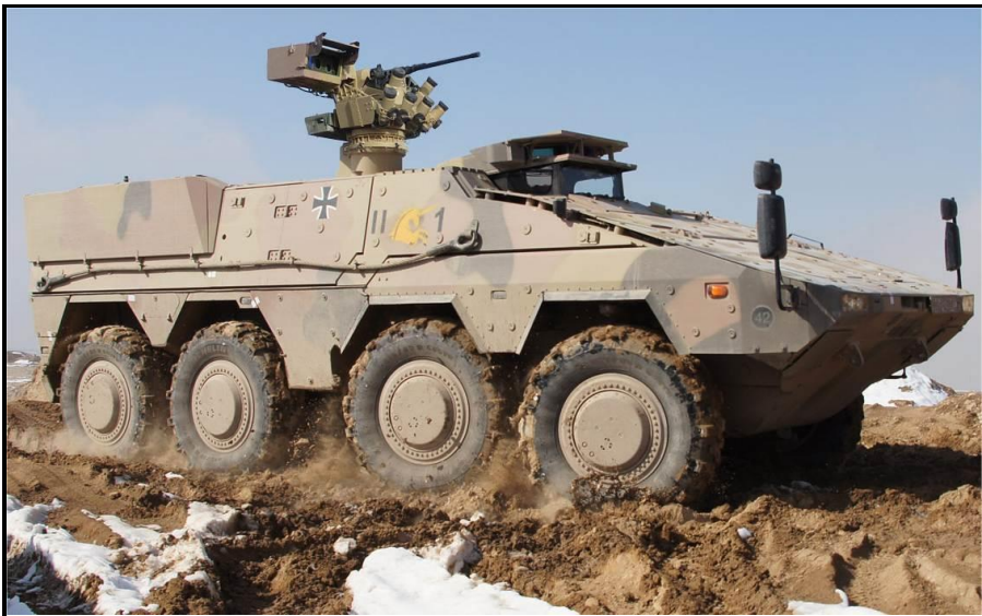
Figure 7: A German BOXER fifth generation APC with FLW-200 RCWS 16 [25]
