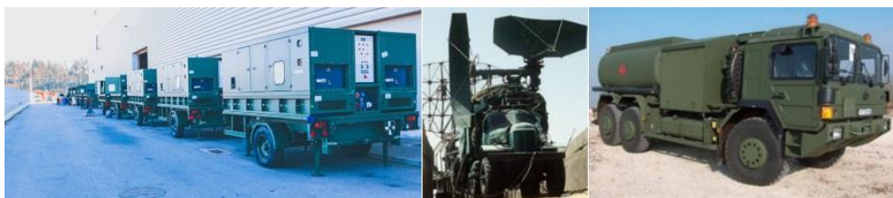
Figure 7. Power generating sets designed for military use 34 , RSP-7(-7T) delivery radio locator station in the middle, 35 Rába fuel transport vehicle and filling wagon on the right. 36
