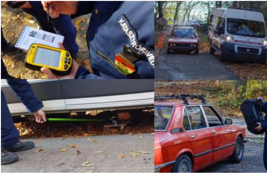
Figure 13: Radioactive source exploration under vehicle, backpack testing at high speed, outdoor site, [own construction]
