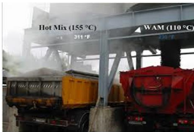
Figure 3. Environmental difference between the production of HMA or WMA [11]
