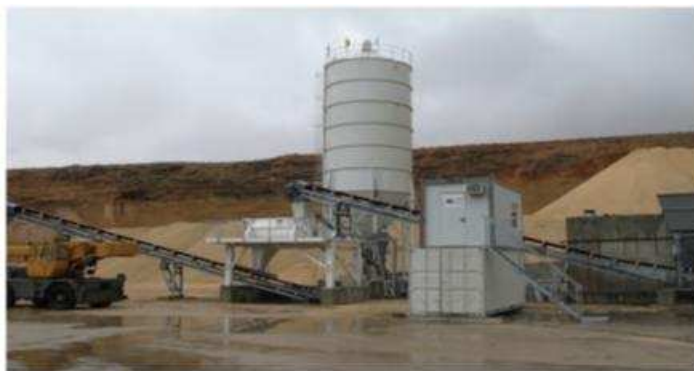
Figure 5. Cold asphalt mixing plant [16]
