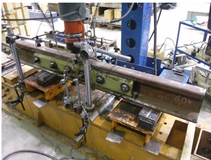
Figure 1. Assemblage for loading the glued insulated rail joint
