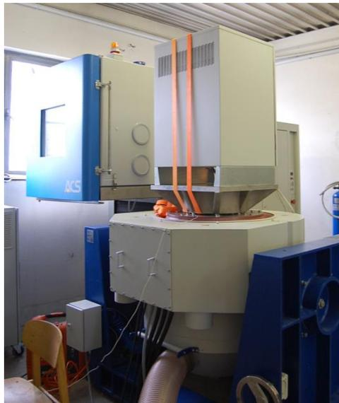
Figure 2. Electro-dynamic vibration system
