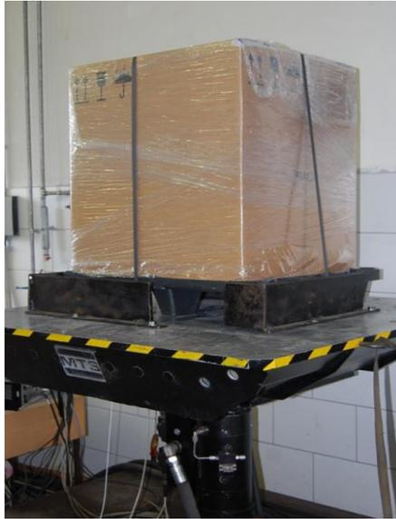
Figure 1. Servo-hydraulic vibration system
