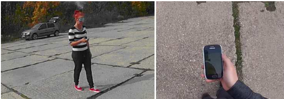
Figure 4. A blindfolded subject during testing (left) and the proper way to hold the device during navigation (right).
