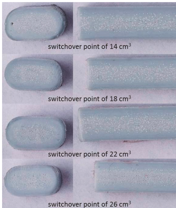
Figure 4. The longitudinal and cross-section of a sample made with different switchover point
