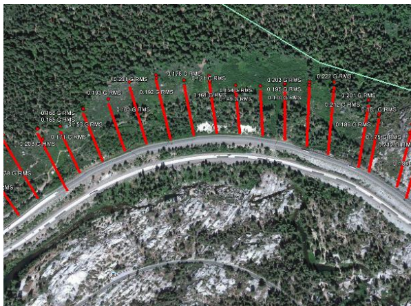
Figure 6. Measured g values imported to Gmaps (Source: own measurement and Lansmont Ltd)
