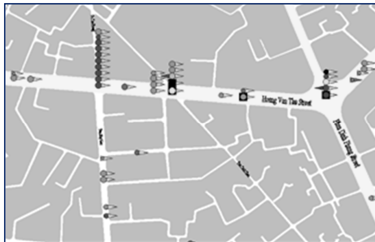
Figure 12. Typical example of Accident Pin Board (APB) of the area under study
