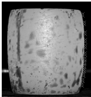
Figure 11: Geometry of the sample No.5. at 23.45 % height reduction. Correlation coefficient: c=0.993
