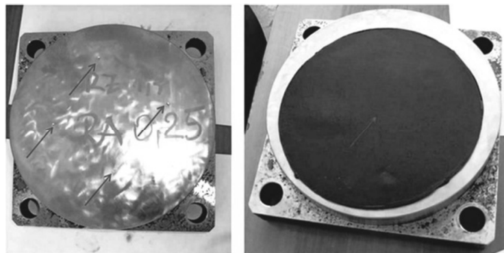
Figure 7. Taking silicone replica of the active surface of the lower upsetting die
