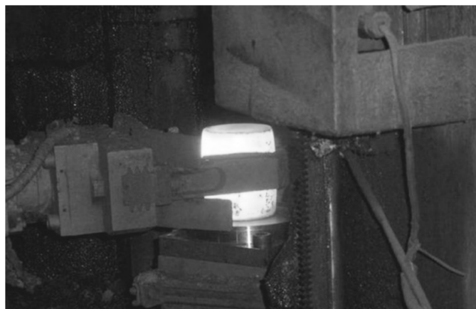
Figure 2. Manipulation of the upset forged part by a robot
