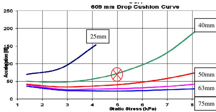
Figure 7. The cushion characteristic of an environmental friendly cushion (cc40 mm thick material at 5 kPa static stress, with 73 g)
