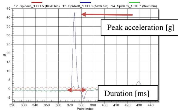
Figure 5. Registered shock during a drop on a packaged product (source: Authors)
