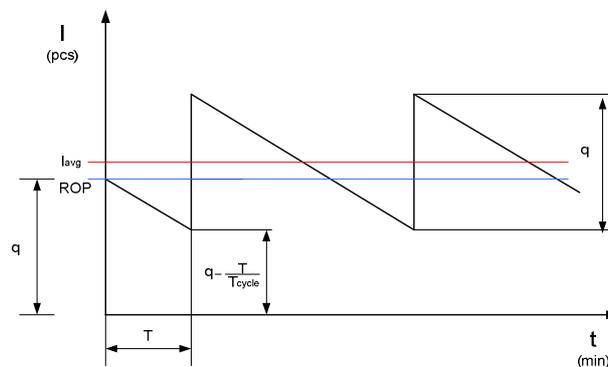
Figure 2. Inventory diagram of single production lines
