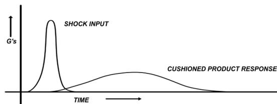
Figure 6. Idealized shock input and cushioned response (source: Authors)
