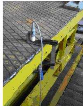
The accelerometer Type B12-500 fixed on the vibration table
