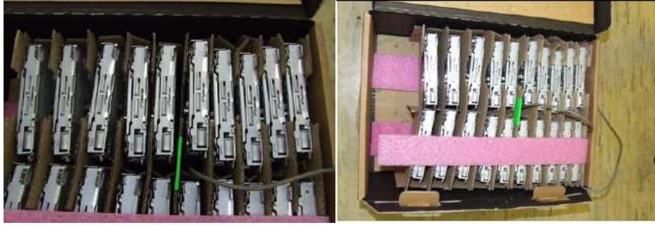
Figure 11. Condition of package after vibration and drop test (source: own photo)
