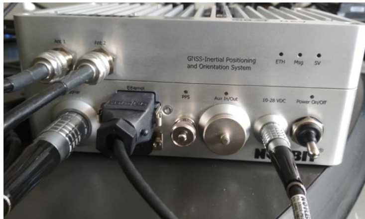
Figure 5 The Sonar Interface Unit (SIU) with the connecting cables
