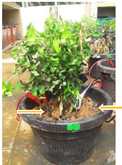
Figure 1. The vertical insertions of electrodes (yellow arrows) into the soil. Plant species ( S. campanulatum ) was positioned in between the electrodes
