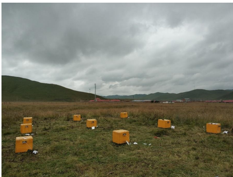
Figure 2. Nitrous oxide emissions measurement using static chamber method at Maqu Grassland Agriculture Research Station of Lanzhou University, China
