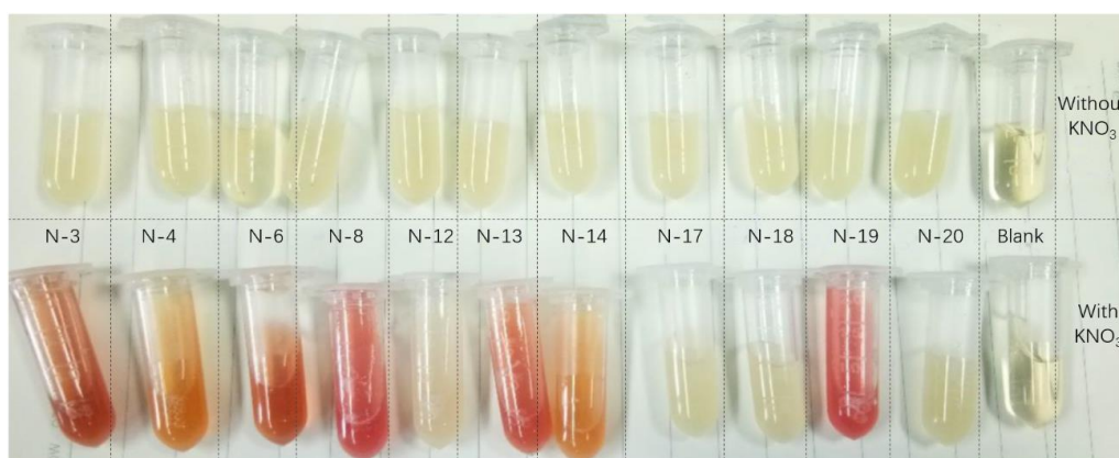
Figure A2. Nitrate reduction test results of 11 colonies whose phosphorus removal rates exceeding 50%
