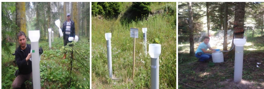
Figure 2. Throughfall, open site and stemflow precipitation collection in Aladağ fir forest
