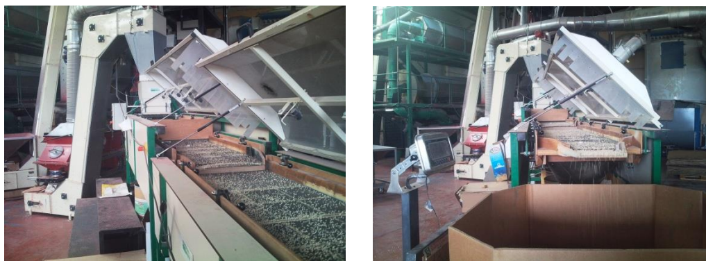
Figure 4. Classification of seeds according to seed sizes in Beta Agriculture and Trade Co. seed processing plant
