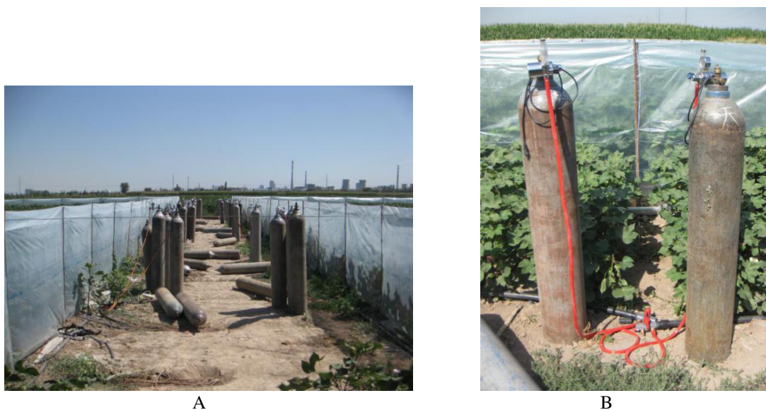
Figure 1. (A) Semi-closed open top artificial climate chamber. (B) CO 2 gas cylinder and pressure reducing valve
