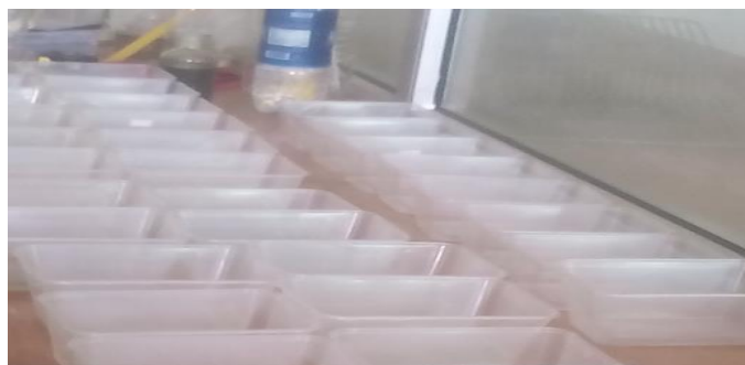
Figure 5. Picture of polyethylene jars arranged for range finding test
