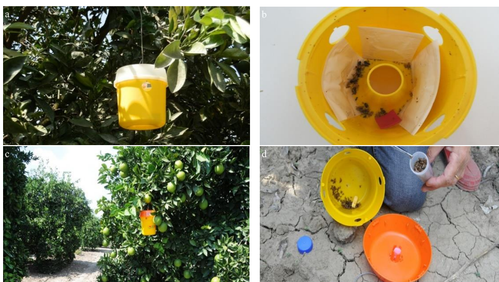
Figure 1. Trapping devices used in the field trials: a, b: Tephti trap with Biolure, c, d: Eostrap with Trimedlure
