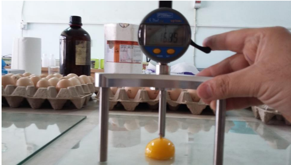
Figure 5. Spherometer used for measure yolk height
