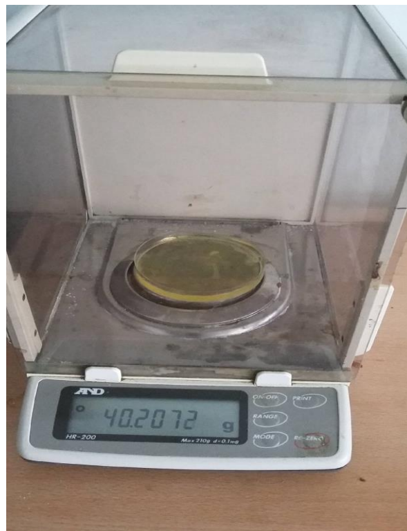
Figure 2. Sensitive electric balance type Mettler Toledo used to measure albumin weight
