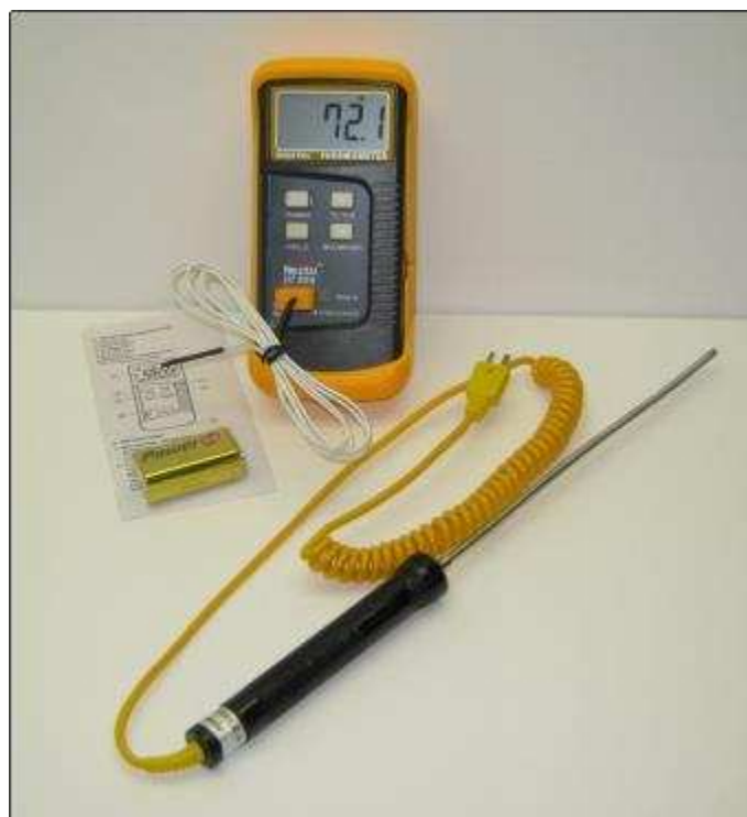
Figure 4. Thermometer digital and thermocouple Type K (Nicety ® DT804)
