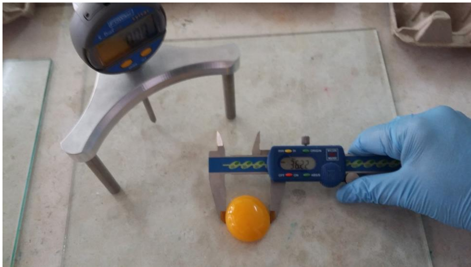
Figure 6. Digital Vernier used for measure yolk diameter
