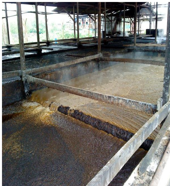
Figure 2. Palm oil mill effluent (POME) sludge gathered from conventional aerobic pond treatment
