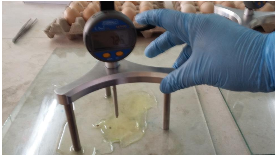
Figure 4. Spherometer used for measure albumin height
