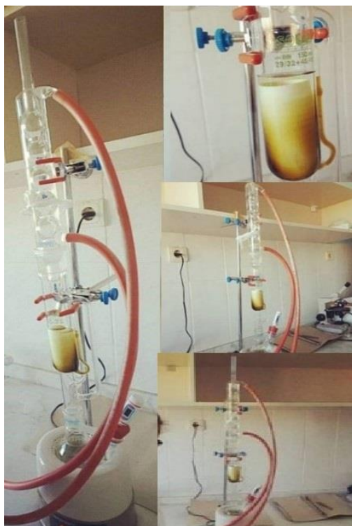
Figure 3. Soxhlet device extraction process
