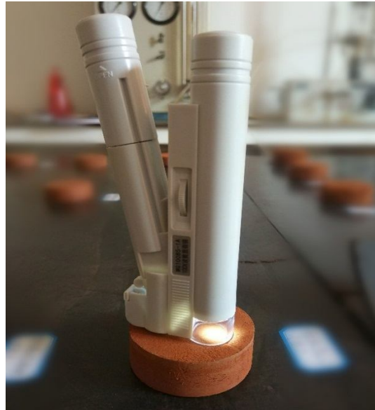
Figure 2. The visualizer of crack width (100x)
