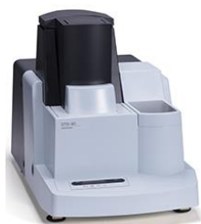
Figure 1. DTG-60 differential thermal-thermogravimetric analyzer
