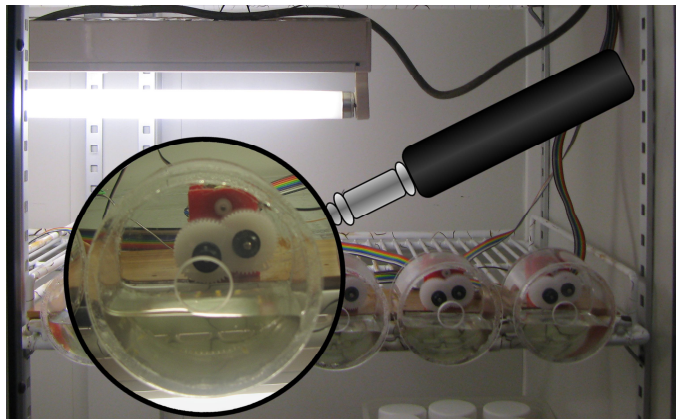
Figure 3. Rotating tumblers filled with filtered lake water, enriched with an appropriate suspension of algae
