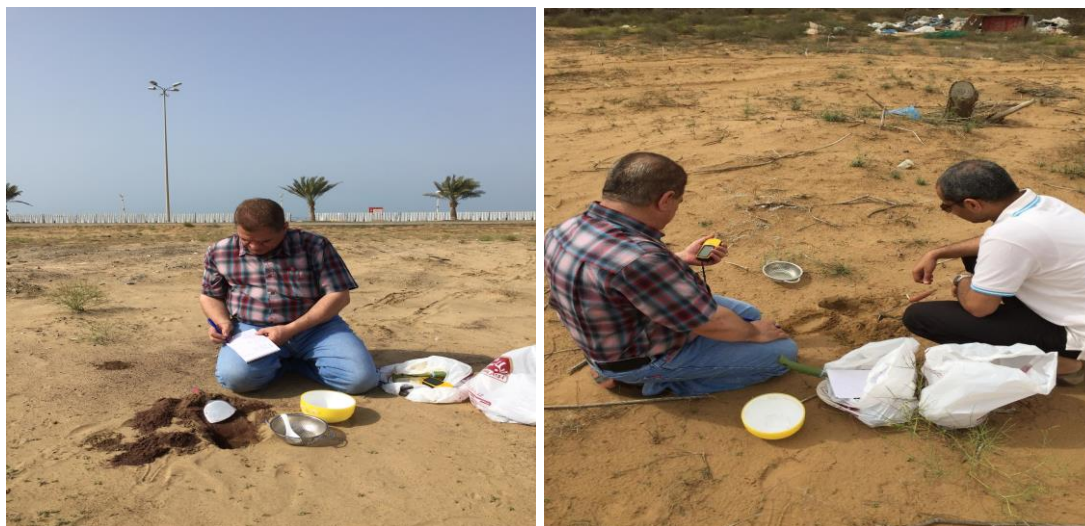
Figure 1. Field photographs clarifying sampling pits and GPS usage for determining sample location attitudes
