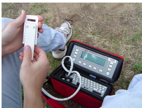
Figure 4. Stomatal resistance measurements were made using an AP4 porometer, Delta-T-Devices®
