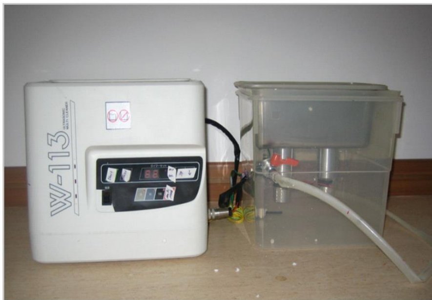
Figure 1. Batch type of ultrasonic reactor was operated at ultrasonic frequencies of 28 kHz, 45 kHz and 100 kHz
