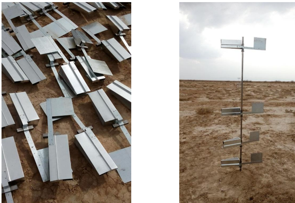
Figure 3. Samplers that were made and installed
