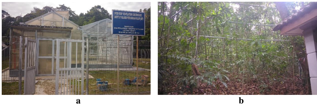
Figure 1. Elevated CO 2 systems (a) open roof ventilation greenhouse system; and (b) free air CO 2 enrichment system
