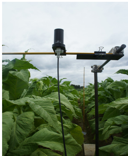
Figure 1. The picture of the self-designed holder for mounting the Remote Cosine Receptor and AccuPAR external sensor
