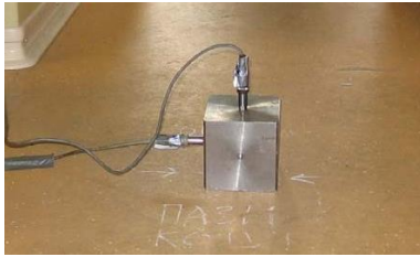
Figure 3 Sensors of acceleration above the main pivot
