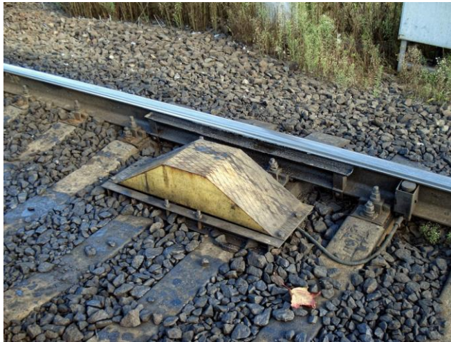
Figure 2 Stationary rail lubricator (SRL-02)
