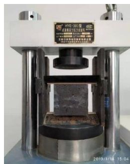
Figure 9 Splitting tensile test layout of concrete specimens
