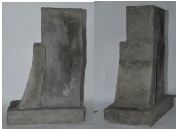
Figure 2 The model of the abutment of the bridge made of cement
