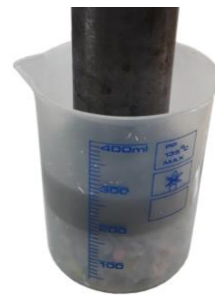
Figure 6 Shredded PET volume reduction test
