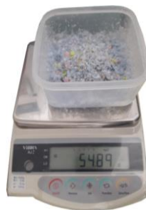
Figure 5 Consistency of the shredded PET bottles
