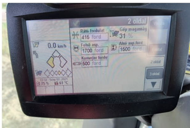
Figure 1: Settings of the harvesting machine
