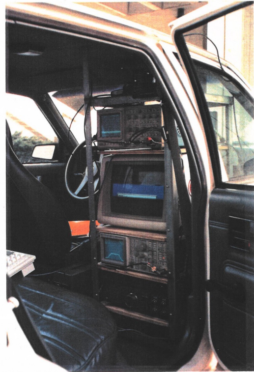
Fig. 9. Full size van converted into a mobile platform to perform noise measurements in the early 1990s [70].
