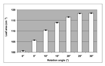
Figure 1: The effect of the angle position of digital camera on the result of leaf area measurements
