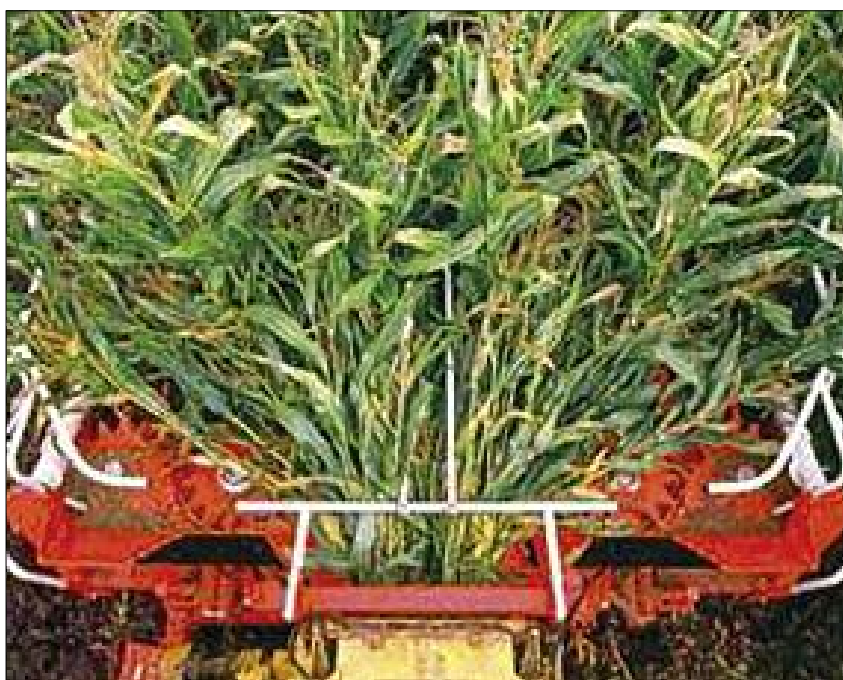
Figure 3: Flow of the cut crop through the special rotary mower (Kemper)
