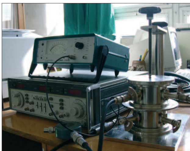
Figure 1: A measuring system utilizing a cavity resonator
