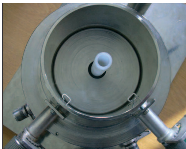
Figure 2: Cavity resonator and sample holder
